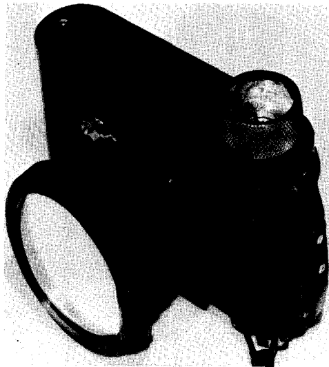
FIGURE 3.—A modified Robot Recorder was used on the Mercury-Atlas 9 flight by Gordon Cooper for experiments in dim-light photography.
