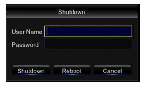
**Shutdown:** Power off the DVR. The unit will shut down immediately and all unsaved settings will be lost.
