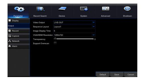
**Video Output:** By default, the DVR automatically selects the output based on the cable connected to the back of the DVR.
