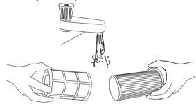
4 Wash both filter and protective mesh under warm water until the water runs clean. Remove excess water by shaking and leave to dry for 24 hours. Reassemble and refit filters to cleaner, only when they are completely dry.
