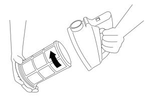
2 Remove the filter assembly from the bin top by rotating the filter. It is advisable to wash the filters after every 5 bin empties.
