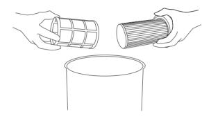
Remove the protective filter mesh from the HEPA filter, then gently tap both filters to release any excess dust.
