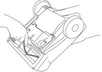
Loop the new belt around the motor and brush channel.
