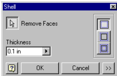
The Shell tool removes material from a part interior, creating a hollow cavity with walls of a specified thickness.
