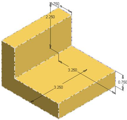
The extrusion's dimensions are now visible. We see that the width is 3.25 units.
