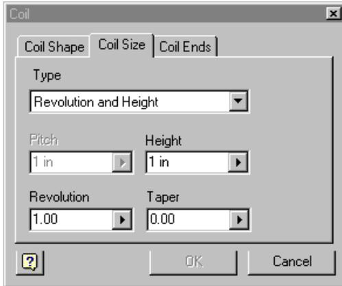
The Coil Size Tab specifies how the coil is created by specifying Pitch, Revolution, and/or Height. Specify two of the three parameters; the third parameter is calculated.
