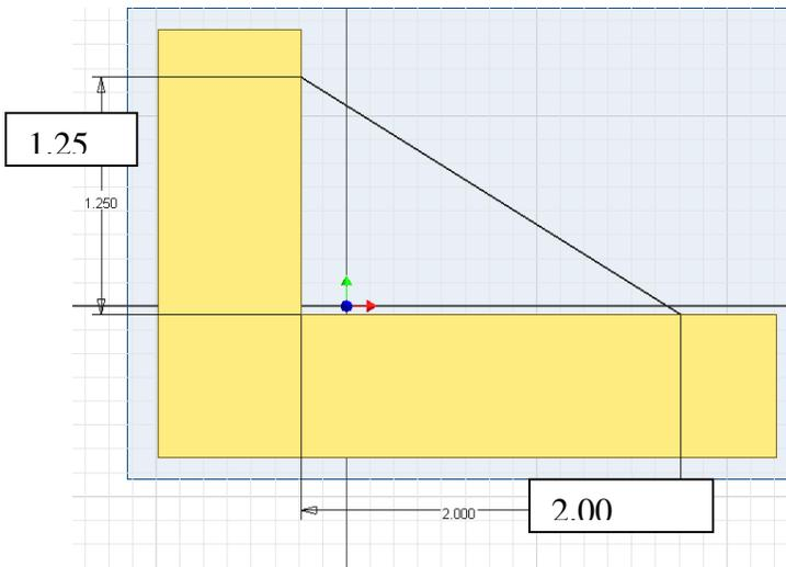
Draw a single slanted line as shown. Add coincident constraints for the horizontal and vertical endpoints and then dimension.
