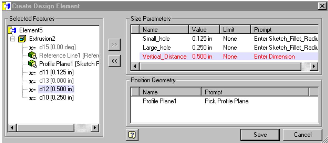
In this example, we have defined the design parameters to be the large hole, the small hole, and the vertical distance between the holes. Notice that the 0.00-inch dimension which forces the holes to line up is omitted at a user-defined parameter. In this way, we can control our design elements and decide which geometries are changeable and which are not.
