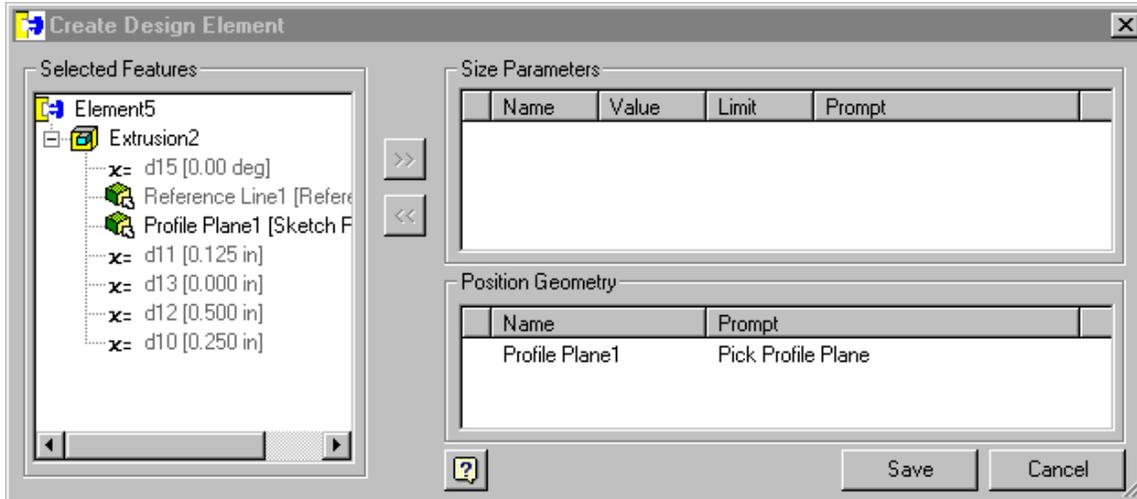
Initiate the Create Design Element command. To select the feature, simply pick it from the Browser. The window with the selected features will fill in as shown.
