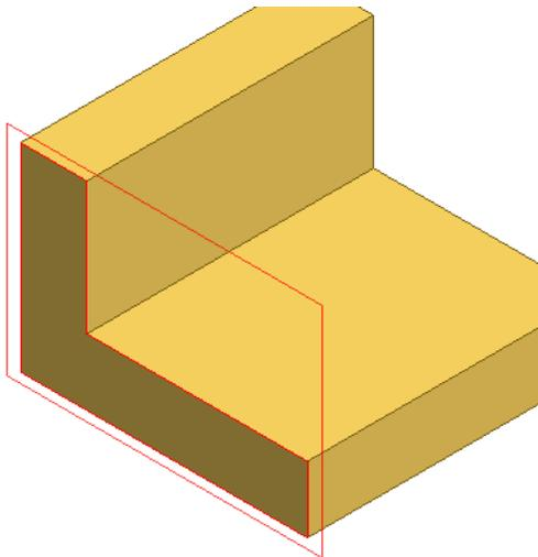
Select the face shown and start dragging the work plane into the part.
