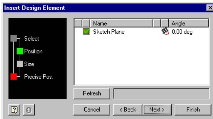
Once the element is selected, the next dialog appears. The user is required to select the plane on the existing model to place the element.
