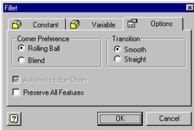
The Options tab sets the corner preference, transition type, and edge chain preference for fillets and rounds. The default settings for these options are correct for most fillet features.
