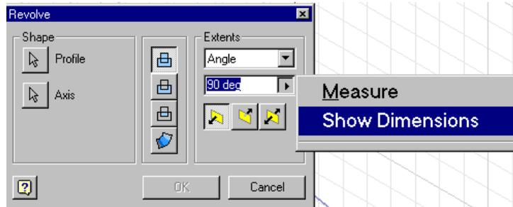
For the angle, you can measure for an angle, show dimensions to help you determine a value or simply type in an angle.
