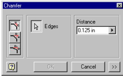
You specify the corner appearance and select edges individually or as part of a chain. All chamfers created in a single operation are one feature.
