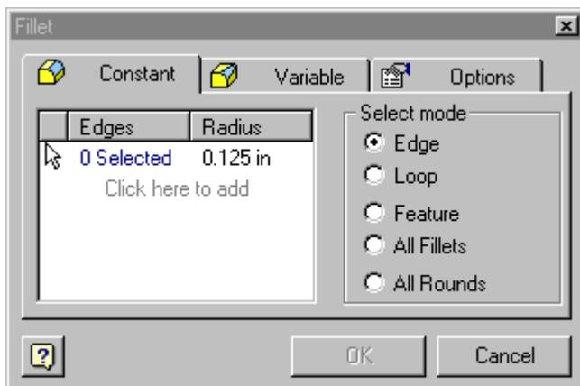
Selecting the Fillet tool brings up the dialog box shown. On the right side, we can set the selection mode of what we want to select. For example, enabling the 'All Fillets' mode, would select all the current fillets defined on the model.
