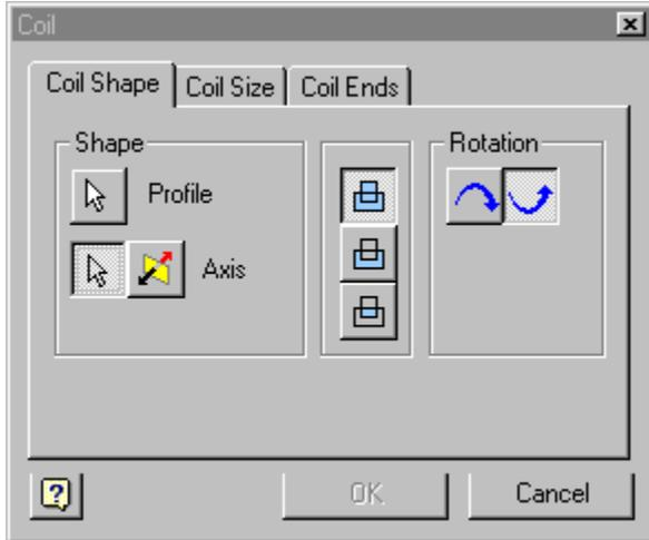
Select the profile we have created. We can adjust whether the coil will be created clockwise or counterclockwise using the Rotation button. Inventor previews our selection so we can decide if the selection is correct. The axis can either be defined using an existing sketch, edge or, if the profile is a circle, selecting the circle profile will automatically set it to the center.
