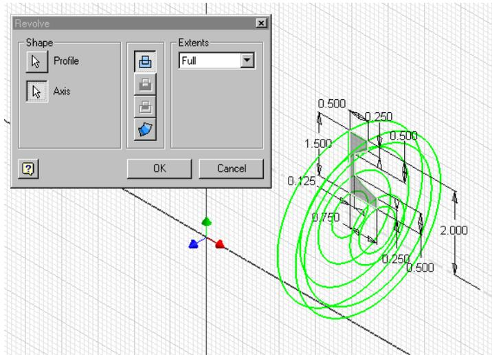
Verify that the correct profile is highlighted. If it is not, left-pick on the profile button in the Revolve dialog box and select the sketch. Because we defined our axis line as a centerline, Inventor automatically knows how to revolve our profile.
