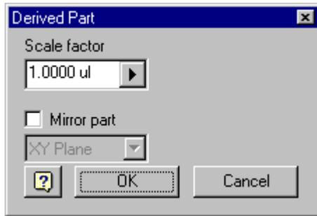
To capture design intent, you can use an Autodesk Inventor part as the basis for a derived part. A derived part is a new part that uses an existing part as its base feature. You can add features to the derived part feature (the base feature), and update it to incorporate changes made to the original part.
