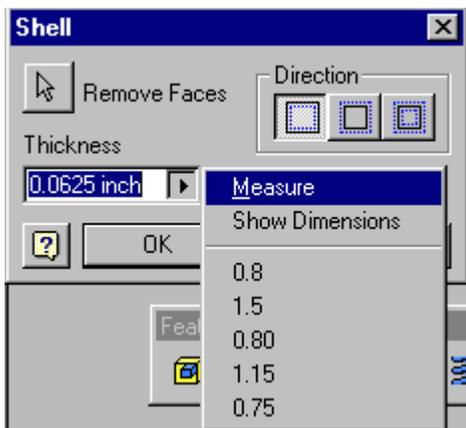
The drop down on the Thickness bar allows you to measure a distance to determine the shell thickness or display dimensions to assist you in determining which thickness value to use. Inventor stores the most common values and displays them to aid you in making a choice.
