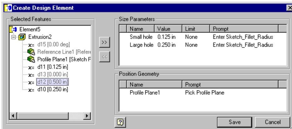
Notice that when a parameter is highlighted, the top double arrow becomes available to insert into the Size Parameters.
