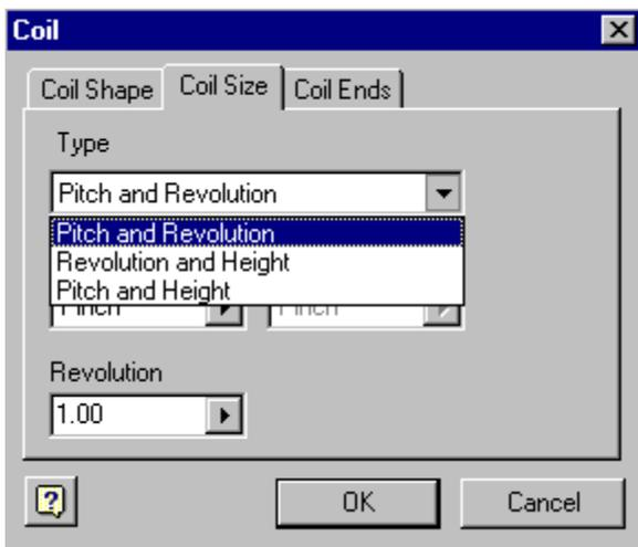
We can define a coil using Pitch and Revolution, Revolution and Height, or Pitch and Height. To modify the values, place the mouse cursor inside the edit box and type the desired value.
