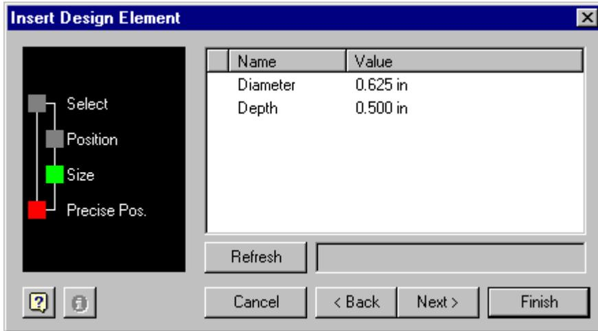
The user is then prompted for the values for the element to be placed. At this time, the user can specify his specifications for the design element.
