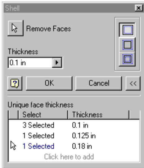
Pressing on the double arrow button located on the lower right of the Shell dialog box enlarges the dialog box, providing the user with the ability to define sides with different thickness values. To remove items from the unique face thickness list, highlight and press the ‘Delete’ key in your keyboard.
