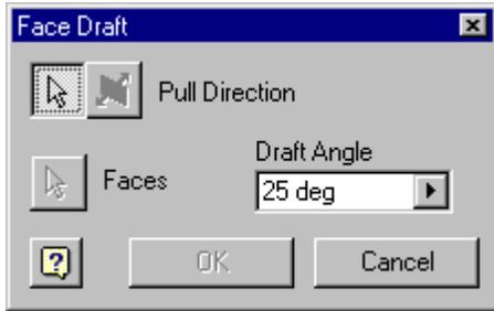
Draft is a taper applied to part faces so that a part can be retrieved from a mold or to cant one or more faces. When designing features for molded or cast parts, you can apply draft by specifying a taper angle for an extrusion or sweep. To add draft to an existing feature or to individual faces, use the Face Draft tool. When applying draft to a face, the relationship between the pull direction and the fixed edge determines the result of the operation.
