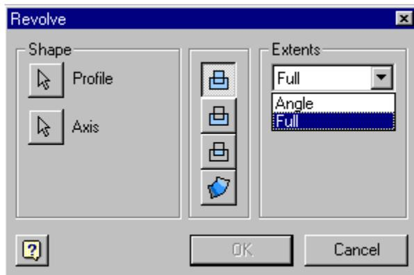
Under Extents, you determine the method for the revolution and set the angular displacement of the profile around a centerline. Click the drop-down arrow to list the extent methods, select one, and enter a value. Revolutions can be a specific distance or can terminate on a work plane or part face.
