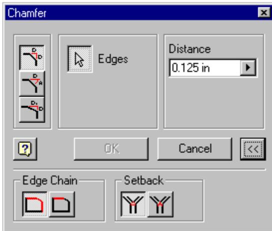
Pressing the double arrow brings up additional chamfer options. The Edge Chain option controls whether the chamfer affects all tangential edges or only the selected edge. The Setback option controls whether or not a setback is added.
