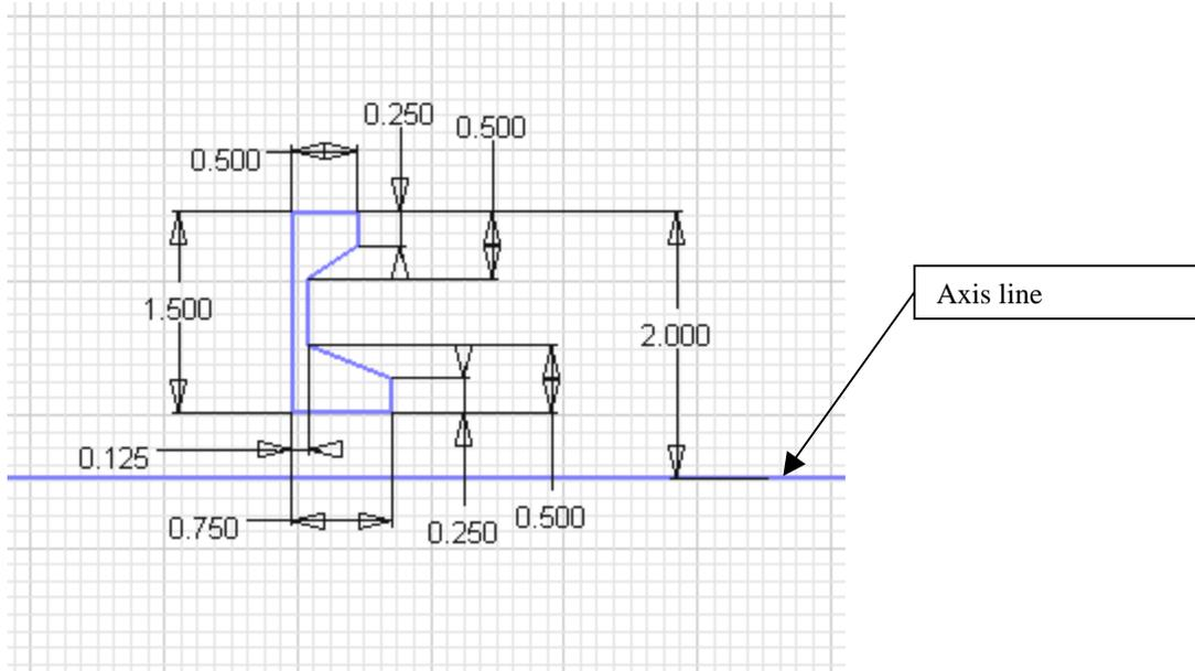
Draw the sketch shown. Note the axis line. This will be used to revolve around. Inventor R4 comes with three line types: Normal, Construction, and Centerline. We can identify the axis line as a centerline by selecting it and then selecting Centerline from the drop down.
