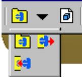
The next section of the Features tool bar contains the Catalog flyout tools and the Derived Component tool.
