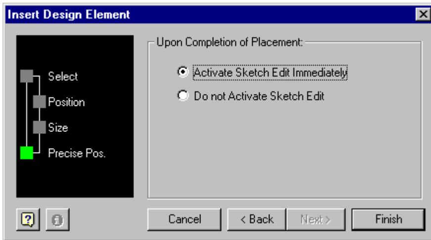
The user is then allowed to set whether to enter Sketch Edit mode immediately upon placement. Entering Sketch Mode allows the user to reposition the element or make further modifications to the basic element.
