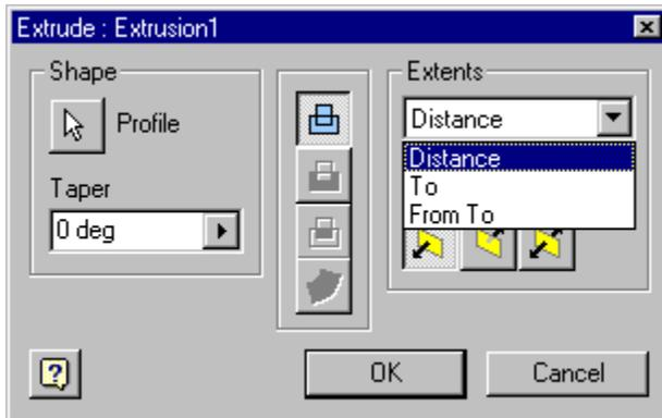
Under the Extents section of the dialog box, there is a drop down that allows you to define how far you want to extrude the profile. Your options are Distance, To, and From To.
