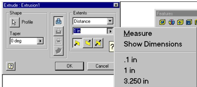
Inventor automatically saves your most common values. You can also measure objects on the fly to determine what value you want to use. You can use the Show Dimensions to select an existing dimension on the model to be used for the feature being defined.
