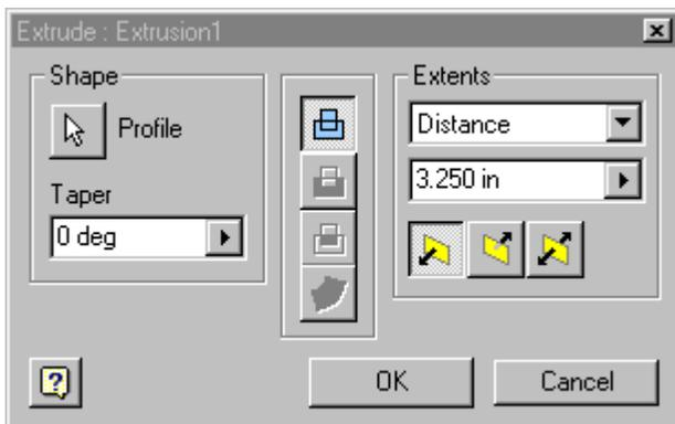
The Shape button selects a profile to extrude. If there are multiple profiles and none are selected, click Profile and then click on one or more profiles in the graphics window.
