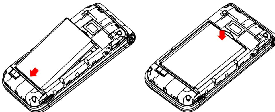
battery with the gold contact points of the compartment. It only fits one way. Press down to position in place.
