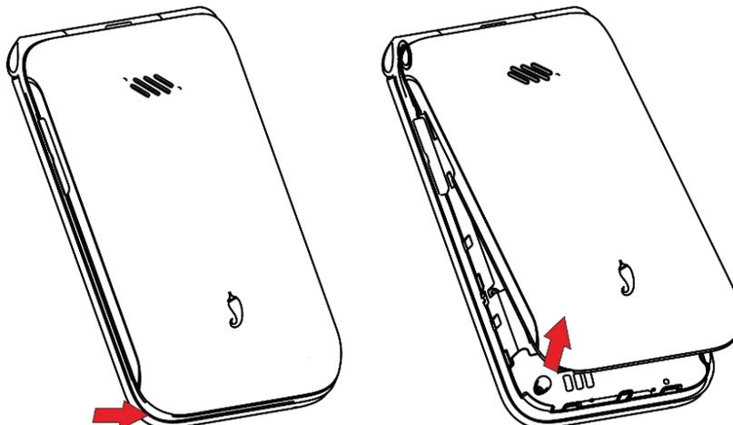
**Step 2.** Remove the battery using your fingernail to lift from the top.
