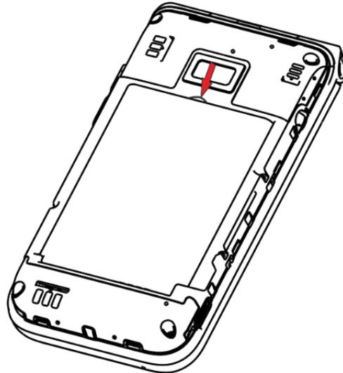
**Step 3.** To insert SIM card ① or microSD card ②, push the SIM card or microSD card into the card slot with the gold-colored contacts facing down.
