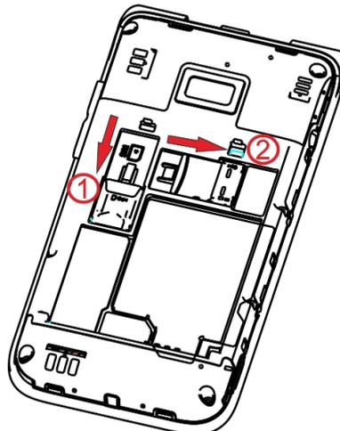
To remove the SIM card or microSD card, press down on the small plastic tab, then slide out the card. Do not use force or any sharp objects.
