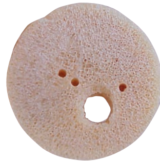
Example of bone removal with standard lag screw
