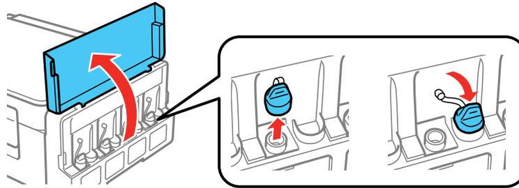
**Note:** Make sure the color of the ink tank label matches the ink color you want to refill, and only remove the cap from that ink tank. Be careful not to spill any ink.
