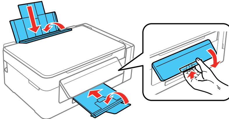
**Caution:** Do not lower the control panel without first squeezing the release bar or you may damage your product.
