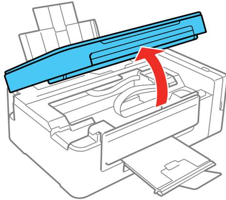
**Caution:** Do not touch the flat white cable inside the printer. Do not lift the scanner unit while the document cover is open.
