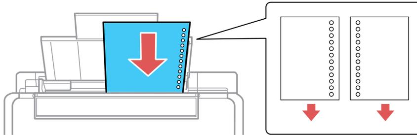
6. Slide the edge guide against the paper, but not too tightly. Then flip the feeder guard back.
